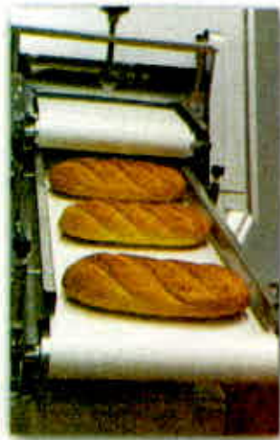
ੳ) Conveyor Belt
