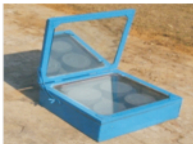
Figure 4.3 Box type solar cooker Figure 4.4 Double reflector solar cooker
