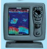
The Echo Sounder is a type of SONAR (Sound Navigation and Ranging) device. It is used determining the depth of the sea bed or detecting objects
