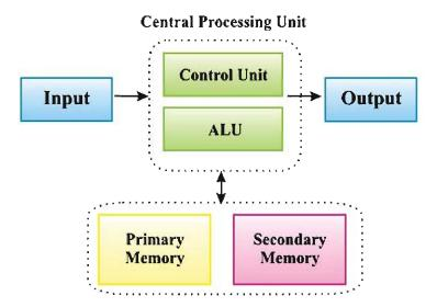
Figure 1.2 : Basic Components of Computer
