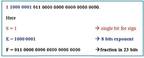
Figure 4.16 : Example of a Number in IEEE Format
