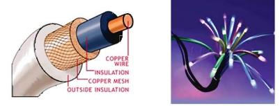
Figure 13.7 : Co-axial Cable and Optical Fiber
