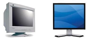
Figure 3.8 : CRT and LCD Monitor
