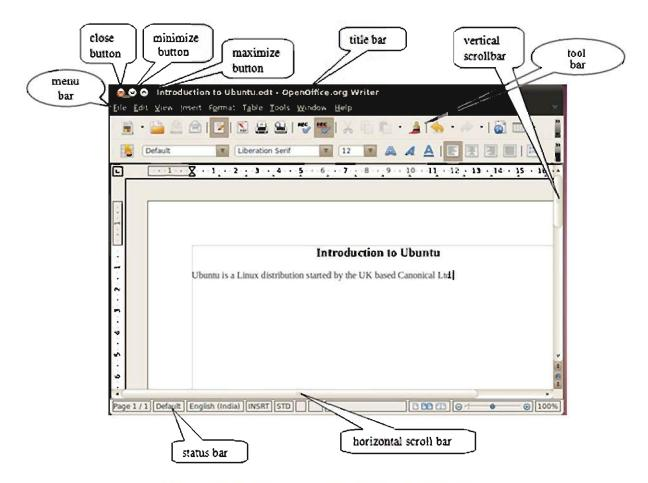
Figure 6.11 : Components of Ubuntu Window
