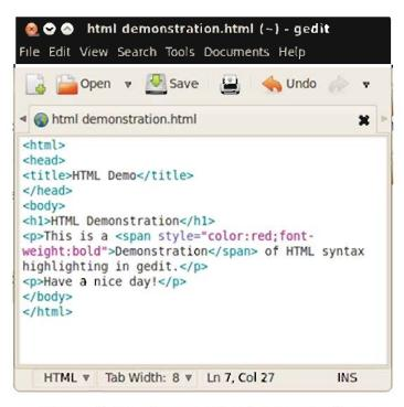
Figure 8.15 : Syntax Highlighting in Gedit
