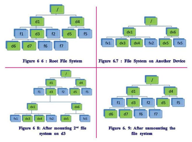
Figure 6.6 shows the root file system. Figure 6.7 shows the file system on another device. Figure 6.8 shows the situation after mounting the file system of figure 6.7 onto the directory d3 of Figure 6.6. The original contents of d3 are now masked and the contents of the file system mounted there appear as if they are the contents of d3. Figure 6.9 shows the situation after unmounting the second file system. The original contents of the directory d3 now become visible again.
