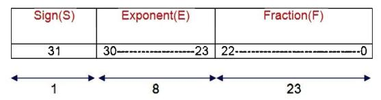
Figure 4.15 : IEEE 32 bit Single Precision Floating Point Number
