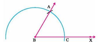
Construction 5: To construct an angle of measure 120°.
