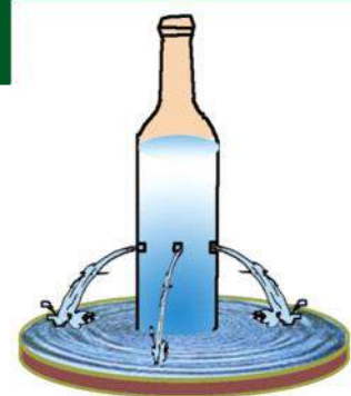
Fig. 3.7 Liquid exerts equal pressure on the walls at equal depths.
