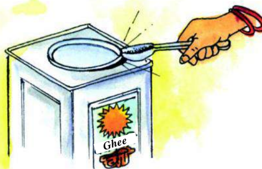
Fig. 11.7 Spoon in the form of a lever
