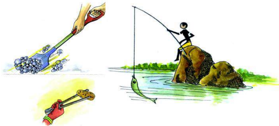
Fig. 11.11 Lever of the Third kind
