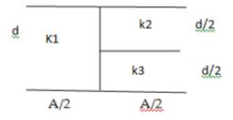
11 You are given an air filled parallel plate capacitor C1. The space between its plates is 2(2011) now filled with slabs of dielectric constants K1 and K2 as shown in C2 . Find the capacitances of the capacitor C2 if area of the plates is A and distance between the plates is d.
