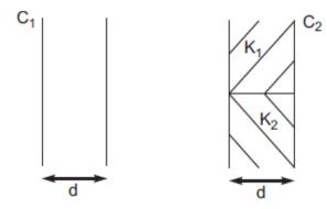
12Two identical parallel plate (air) capacitors C1 and C2 have capacitances C each. The<br/>between their plates is now filled with dielectrics as shown. If the two capacitors still<br/>have equalcapacitance, obtain the relation between dielectric constants K, K1 and K22(2011)
