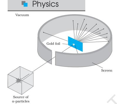
FIGURE 12.1 Geiger-Marsden scattering experiment. The entire apparatus is placed in a vacuum chamber (not shown in this figure).
